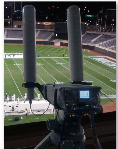
Receiver with antennas on tripod
