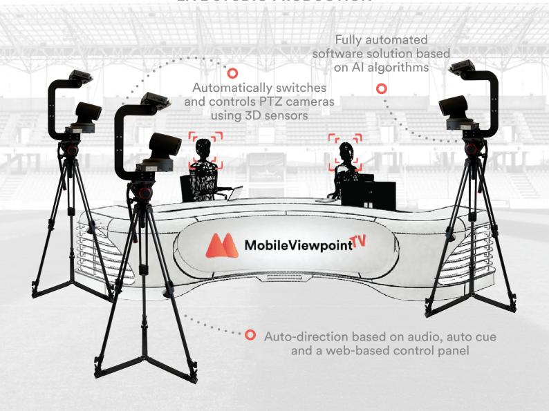
VPilot from Mobile Viewpoint is an innovative production solution that enables broadcasters to create completely automated live news programming without the need of a cameraman or director. Control over three cameras, a switcher and a graphics engine enables vivid and accurate capture of any interview or news production.
